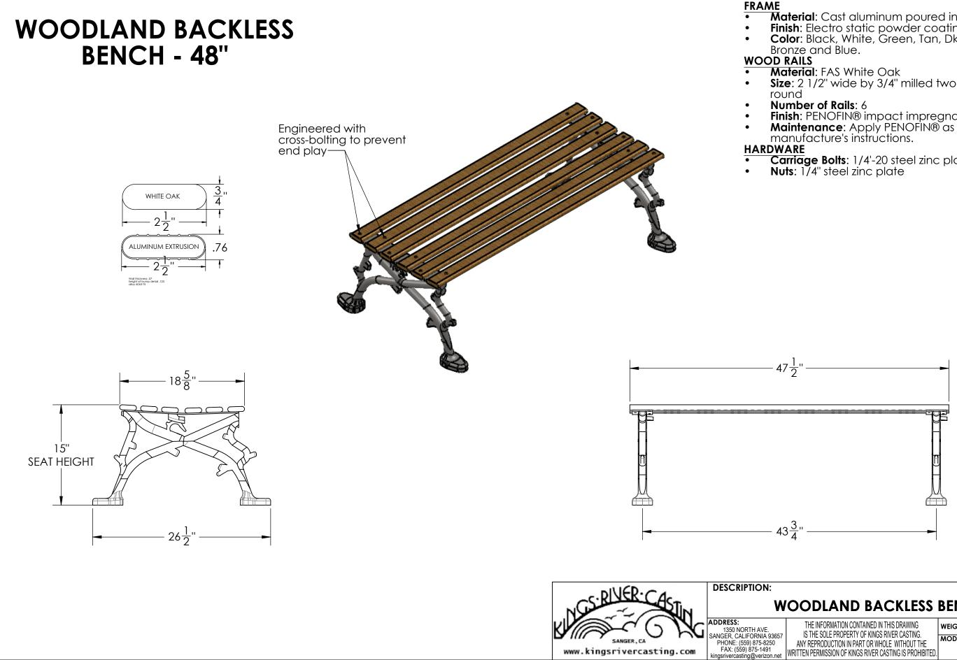
**Material**: Cast aluminum poured in permanent molds **Finish**: Electro static powder coating **Color**: Black, White, Green, Tan, Dk. Brown, Dk. Green,
