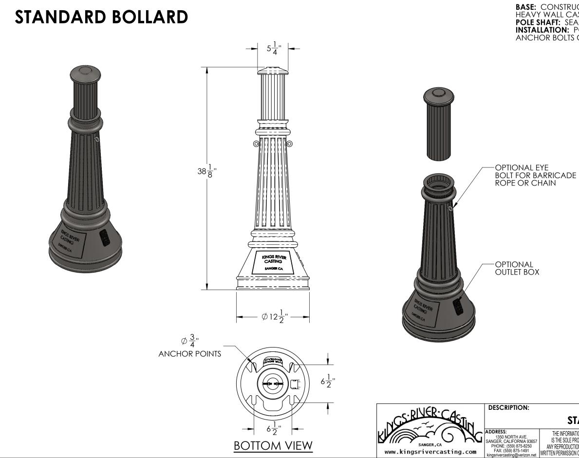
**BASE:** CONSTRUCTED OF DURABLE, CORROSION RESISTANT, HEAVY WALL CAST ALUMINUM. **POLE SHAFT:** SEAMLESS EXTRUDED ALUMINUM. **INSTALLATION:** POST ARE BASE-MOUNTED WITH FOUR ANCHOR BOLTS CONCEALED INSIDE BASE.
